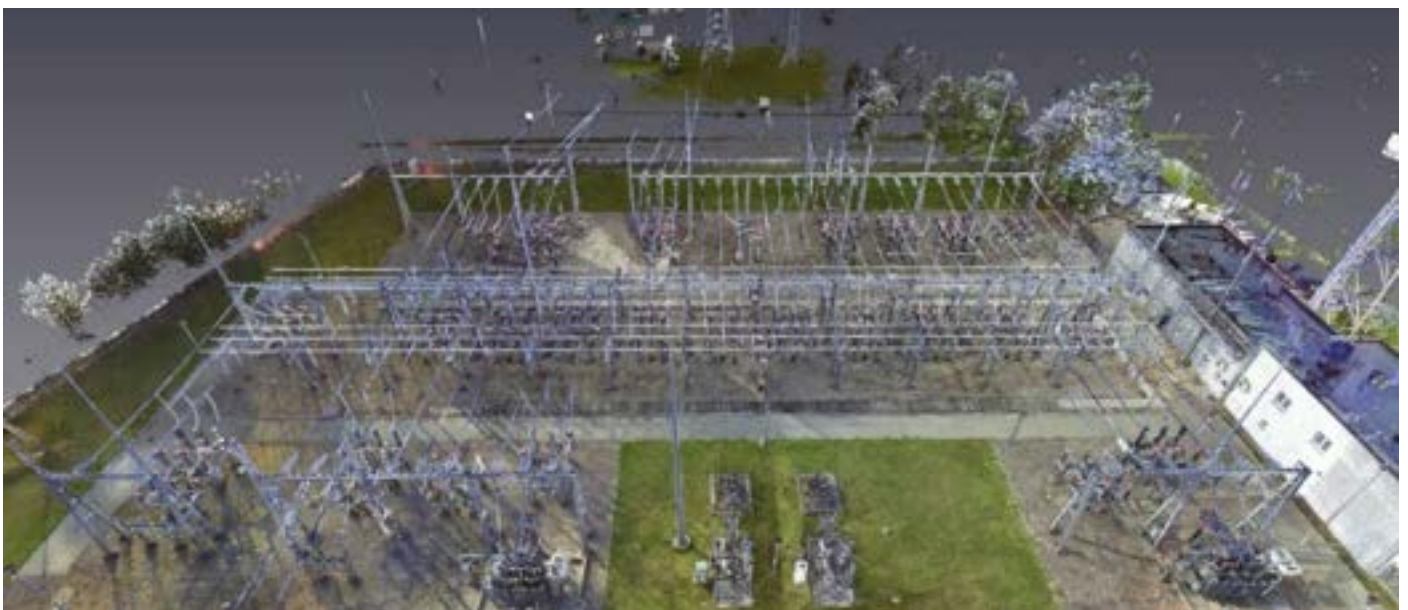
FIG. 3. POINT CLOUD OBTAINED FROM PNIĘWY SUBSTATION MEASUREMENTS
